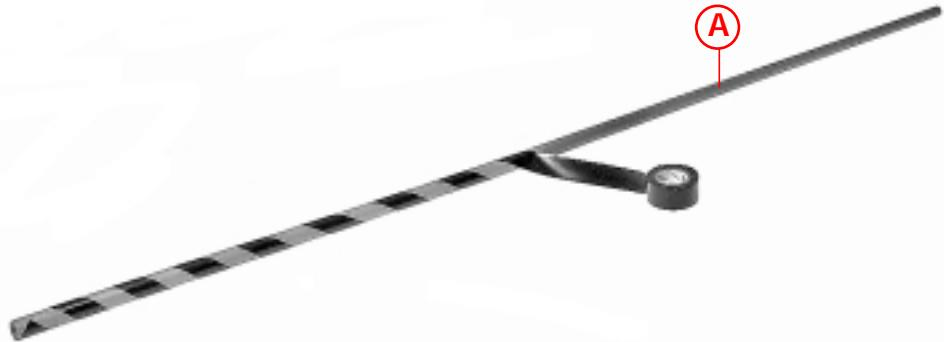
Unroll the insulating tape from the bottom to the top. The distance between the insulating tape stripes is appr. 20 mm.
